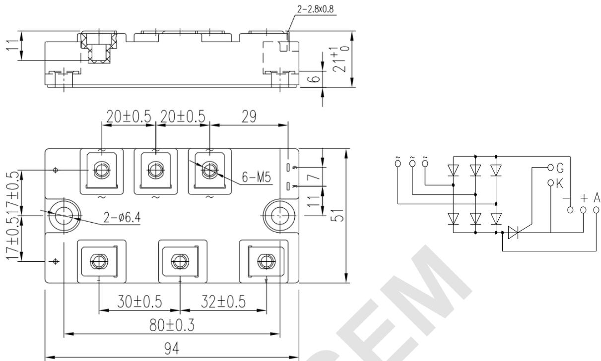
Unmarked dimensional tolerance: ±0.5mm
